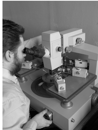
Figure 2. The post graduate student performs his research work of SOI CMOS MOSFETS using probe station.
