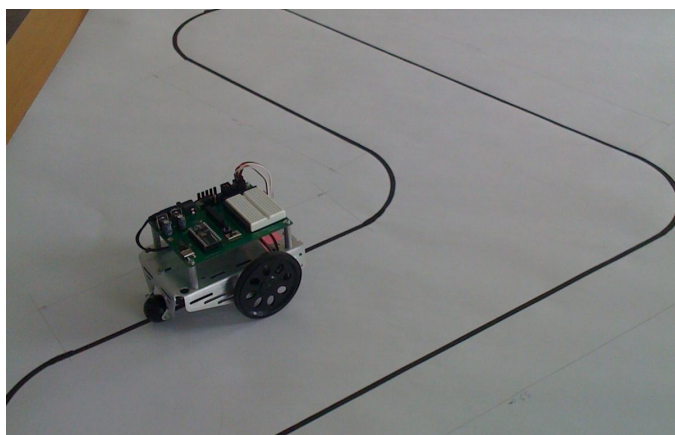
Figure 2. Robot following a predefined path along the black line
