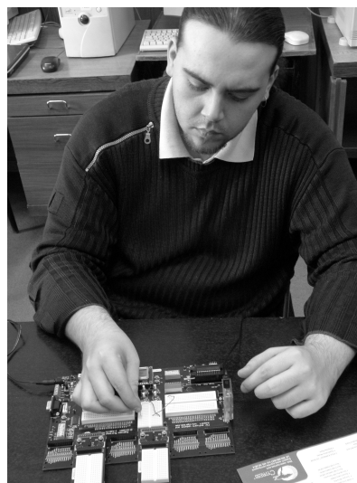
Figure 4. The student performs his term work using CYPRESS development board with CY8C29466-24PVXI microcontroller.
