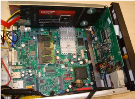
Figure 4. The Car PC comprises off-the-shelf components only.
