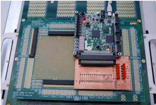
Figure 4. The Interface board and FPGA board connected to the testhead.
