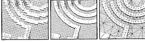
Fig. 5 Detail of a planar coil mesh. From left to right: staircase, conformal hexahedral, tetrahedral.
