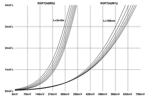
Figure 2. Transconductance characteristic for short and long channel devices.
