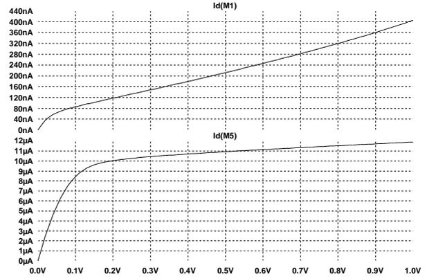
Figure 1.  $I_D$ - $V_{DS}$  Curves of MOS transistors with aspect ratio of 3 and  $L=100\text{nm}$  (up) and  $L=2\mu\text{m}$  (down).
