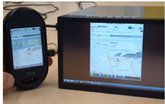
Figure 1. Car PC receives navigation data from a mobile device.
