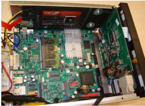
Figure 4. The Car PC comprises off-the-shelf components only.
